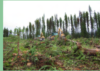
An active harvesting operation using low ground pressure skidders to reduce soil disturbance.
