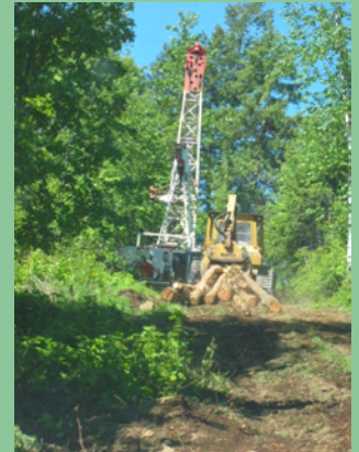
On steep ground cable harvesting systems are used like this grapple yarder operated by Hubschers in Shady Creek. Such cable systems minimize soil disturbance while logging steep ground.
